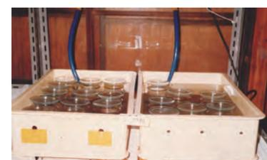
Plankton, fish eggs and larvae samples during the breeding test at higher water temperatures (in 1979)
