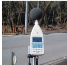
Survey of surrounding environment at the site for environmental assessment (noise level measurement of traffic with an integrating sound level meter) (2002)
