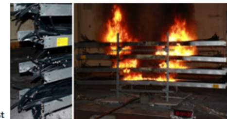
Cable tray fire test
